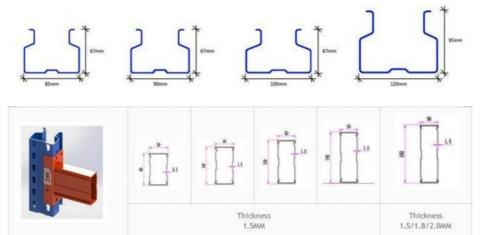
Beam consist of hollow profiles with beam end connectors welded to each end for connection to the uprights. Beam end connectors are available with 3 or 4 pins. The beams have electrostatic epoxy powder coating (standard finish orange RAL 2004). Safety pins can also be used to prevent the beam from unhooking.
